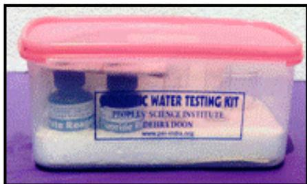
The kits are compact, portable and can test 40 samples of water. Tests for specific parameters can be added at user's request
